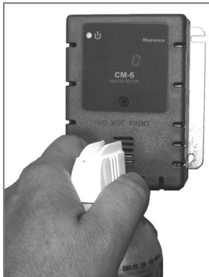
3. Wait for a few seconds. The digital display should climb indicating the increased CO concentration at the sensor confirming a pass of the quick test.
